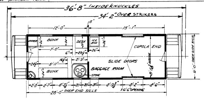
NOTE: CONVERTED FROM STANDARD 28' CABOOSE (BUILT 1923) DIAG. 32 TO BAGGAGE CABOOSE
