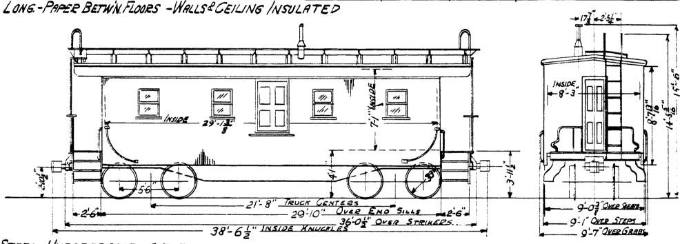
STEEL UNDERFRAME A 5653 BETTEN PORF TRUCKS WITH ELLIPTIC STEEL FRAMING A 5654 SPRINGS ONLY STEEL ROOF A 5444 ELEVATION DRG. HIB7 PLAN - DRG. HISI
