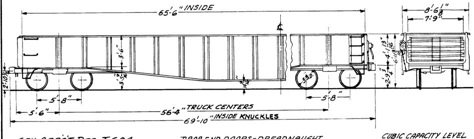
GEN. ARRG'T. DRG. T 604 DROP END DOORS-DREADNAUGHT COUPLERS-A. A.R.TYPE"E"ROTARY, 61/4X8" DROP END MECH. - WINE DRAFT GEAR-PEERLESS H-I-B2.
